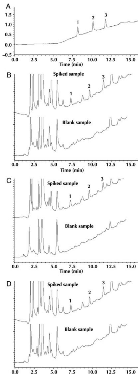
**Figure 5.** The chromatograms of the standard solution (A), porcine blood (B), human blood (C), and white mouse blood (D). The concentration of the analytes in the standard solution and the spiked samples was 0.05  $\mu\text{g}/\text{mL}$ : (1) SDZ, (2) SMR, and (3) SMZ.
